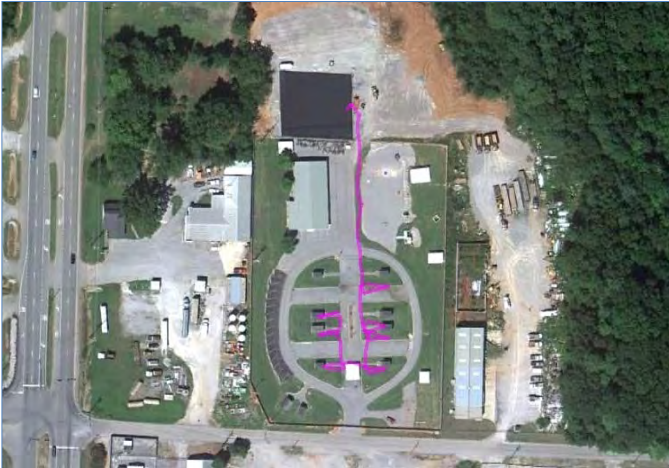
GPS enabled Gas-Rover survey at Leak City, Athens, Alabama 9/12/2011
